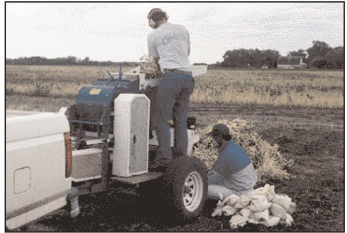
Technicians, using a stationary thresher, harvest dry bean lines from a test plot.
