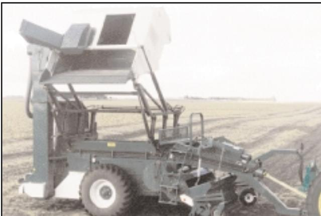
An adjustable vacuum system will remove and separate any foreign material and fines from beans. The bucket elevator will safely deliver the product into an 8,800 lb. capacity dump bin.
